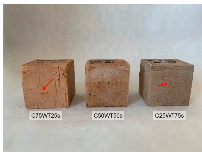
Figure 9. Micro fractures (evidenced by arrows) in some samples cured during the summer season.
